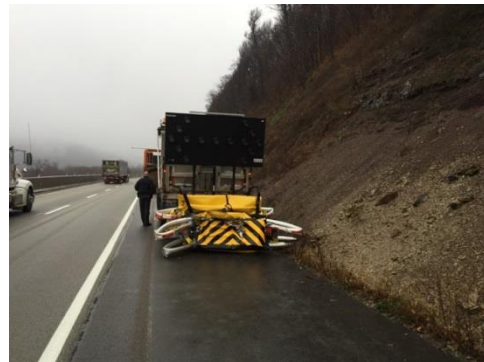
Truck mounted attenuator struck by a commercial vehicle
